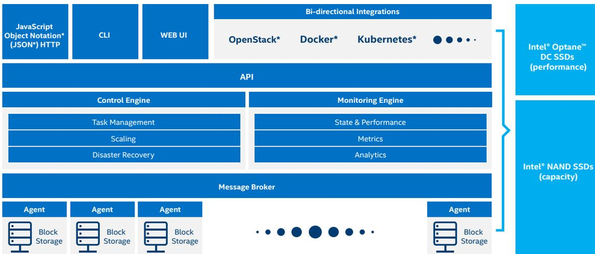
Figure 1. PROZETA BlackStor\* architecture diagram
